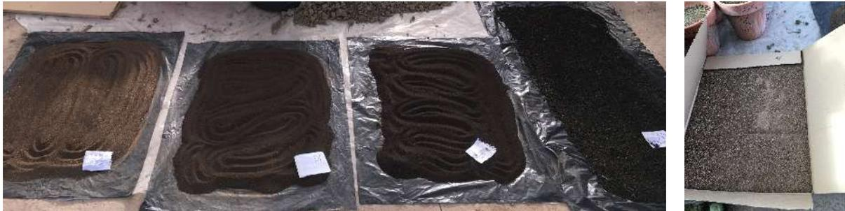
Fig. 2 Dried and sieved soil mixed with the magnetite tracer. The darker mixtures denote higher magnetite concentration.
